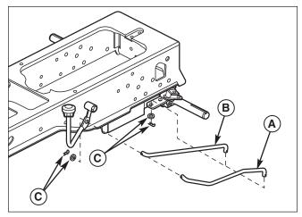
Figure 1. Replace Differential Lock Rod
